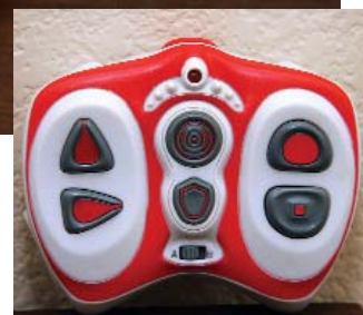
Blazor IR controller. Top center button starts Search & Destroy Mode; mid-center, Guard Mode. Clockwise, from upper left: Forward, Screech/Growl, Stop & Turn right.
