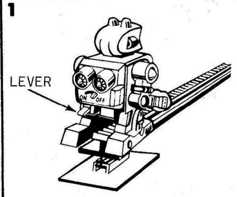
TO MAKE DING-A-LING WALK, SLIDE ONTO ANY STRAIGHT SECTION OF A SPACE SKYWAY SET (SOLD SE-PARATELY). BE SURE LEVER IS IN THE BOTTOM POSITION, AS SHOWN.
