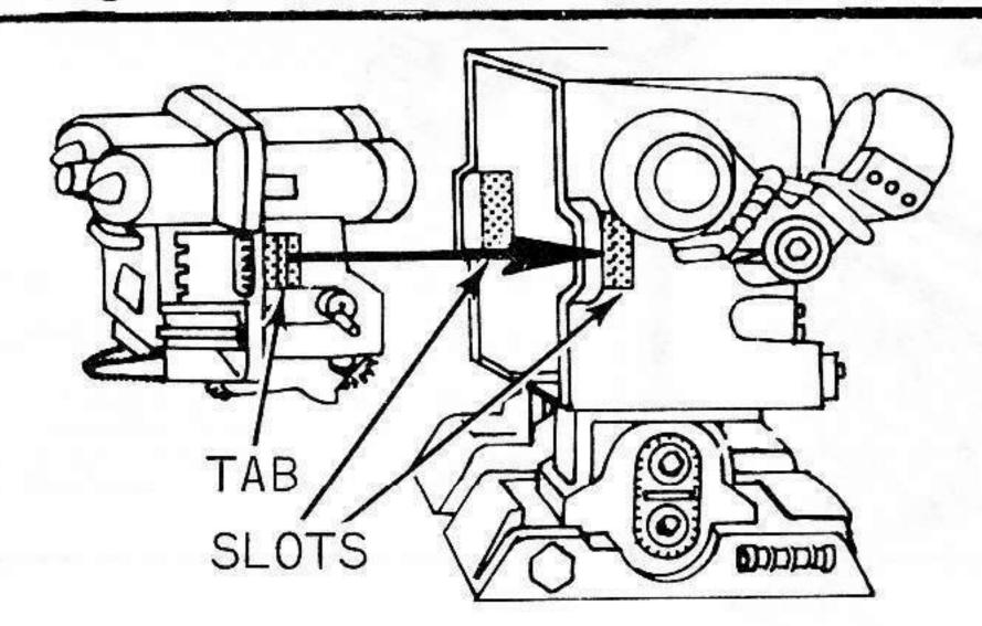
TO INSERT POWER PACK, HOLD AS SHOWN AND PUSH ALL THE WAY IN UNTIL IT CLICKS INTO PLACE. BESURE TABS OF POWER PACK FIT INTO SLOTS IN DING-A-LING, AS SHOWN.
