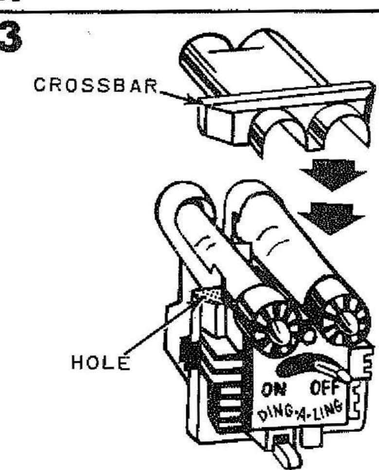
TO PUT ON BATTERY COVER, FIT CROSSBAR INTO HOLES IN POWER PACK AND SNAP COVER INTO PLACE.
