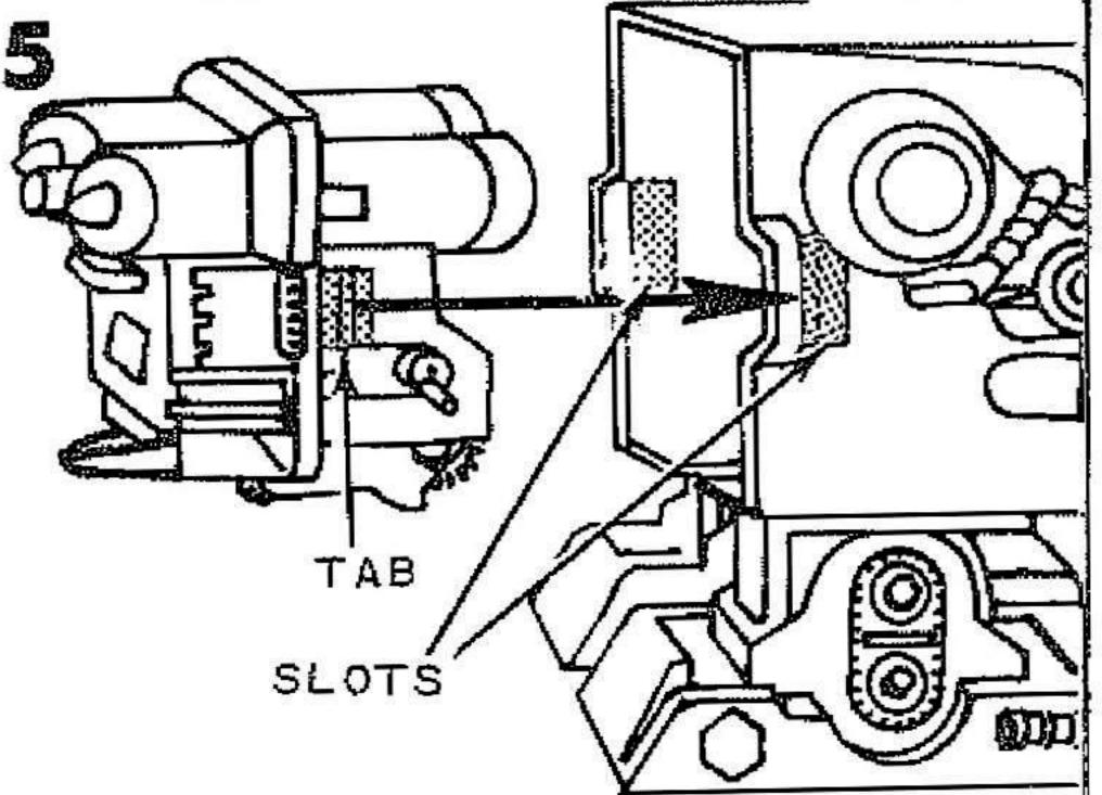
TO INSERT POWER PACK, HOLD AS SHOWN AND PUSH ALL THE WAY IN UNTIL IT CLICKS INTO PLACE. BE SURE TABS OF POWER PACK FIT INTO SLOTS IN DING-A-LING, AS SHOWN.
