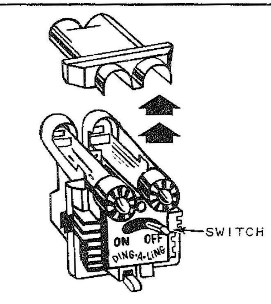
BE SURE SWITCH ON POWER PACK IS OPERATE UNLESS BATTERIES ARE IN THE "OFF" POSITION. LIFT OFF INSERTED PROPERLY AND BATTERY BATTERY COVER, AS SHOWN.
