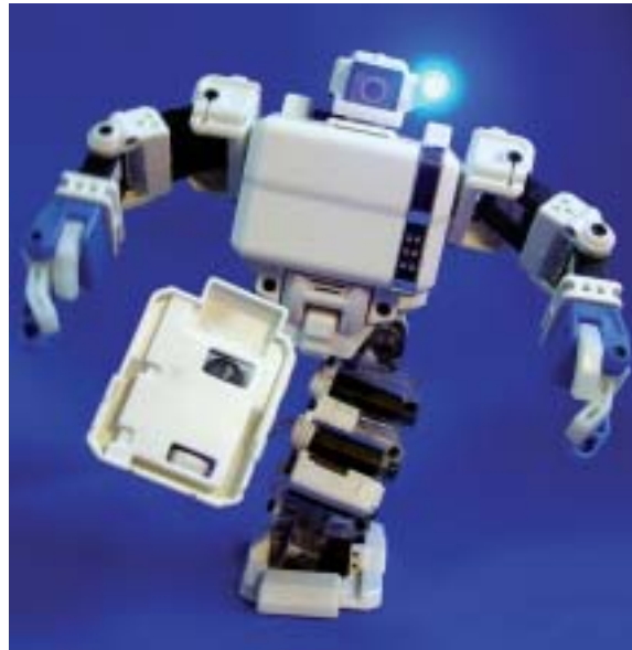
i-SOBOT is equipped with two head mounted LEDs that indicate his operating modes and his moods. Many of the robot's actions are soccer moves, including nice goal kicks by each foot. Notice how the robot shifts its center of gravity over the left foot during the kicking motion using the gyro feedback to maintain perfect balance.
