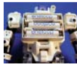
The battery cover is held in place with two screws. For power, the robot uses three AAA eneloop rechargeable batteries, or standard AAA alkaline batteries. The speaker is mounted in a cavity directly below the batteries and provides surprisingly good sound quality.
