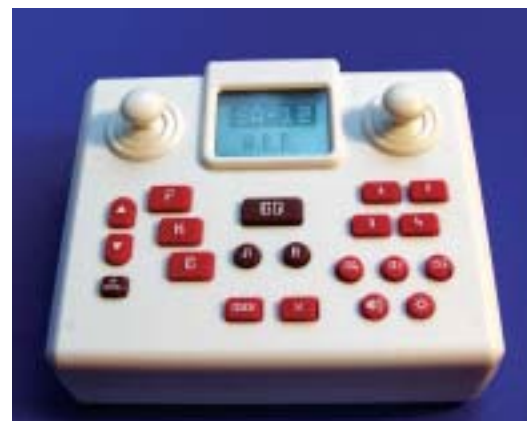
The i-SOBOT remote control has great functionality. The LCD display is invaluable when creating complex programs for the robot.
