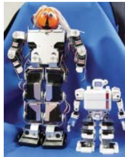
i-SOBOT stands next to a KONDO KHR-1, the original humanoid robot kit first offered for sale three years ago. Both robots feature 17 degrees of freedom, and note the significant difference in size.
