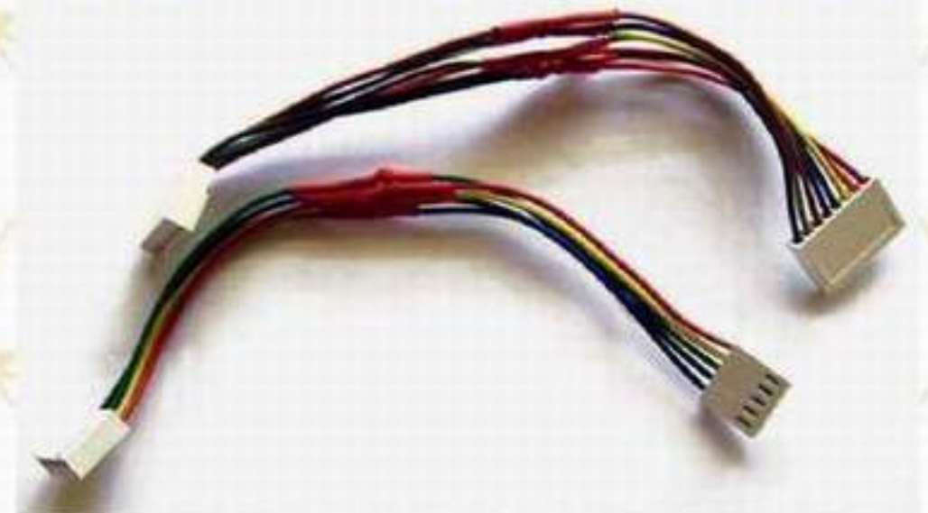
Harness #1 & #2 To Robot Circuit Board
