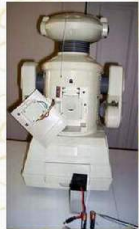
33. Open the rear door and install the large 6 V 4 AH DC rechargeable battery, the two small AA battery's and the battery retainer and close the door.
