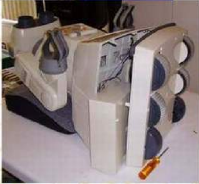
31. Join the bottom base to the housing and install the draw to the robot.
